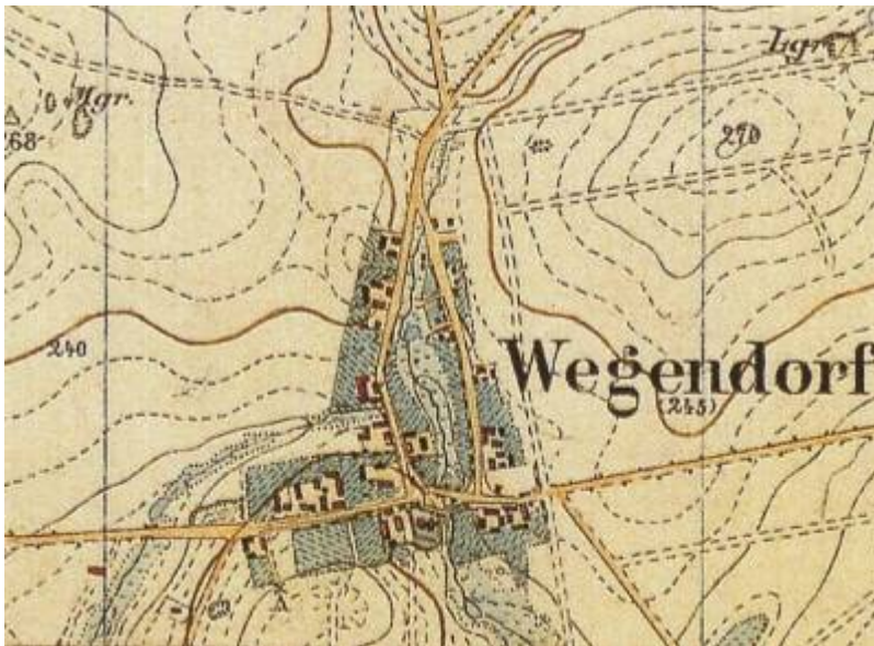
Fig. 13: Indicating elevation contours on a map
