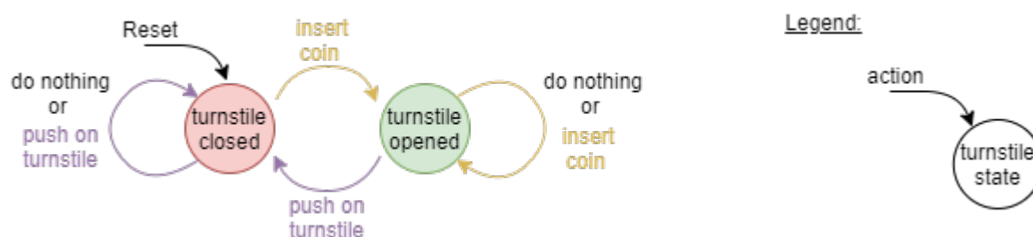
Fig. 12: State Transition Diagramm of the Entrance Control for Toilets
